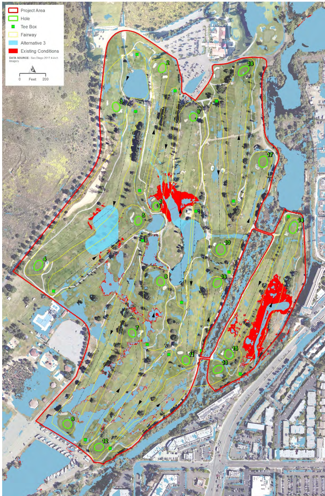
Figure 3-8 Preferred Alternative vs. Existing Conditions, West Hills 100-year 24-hour, Post Event Inundation
