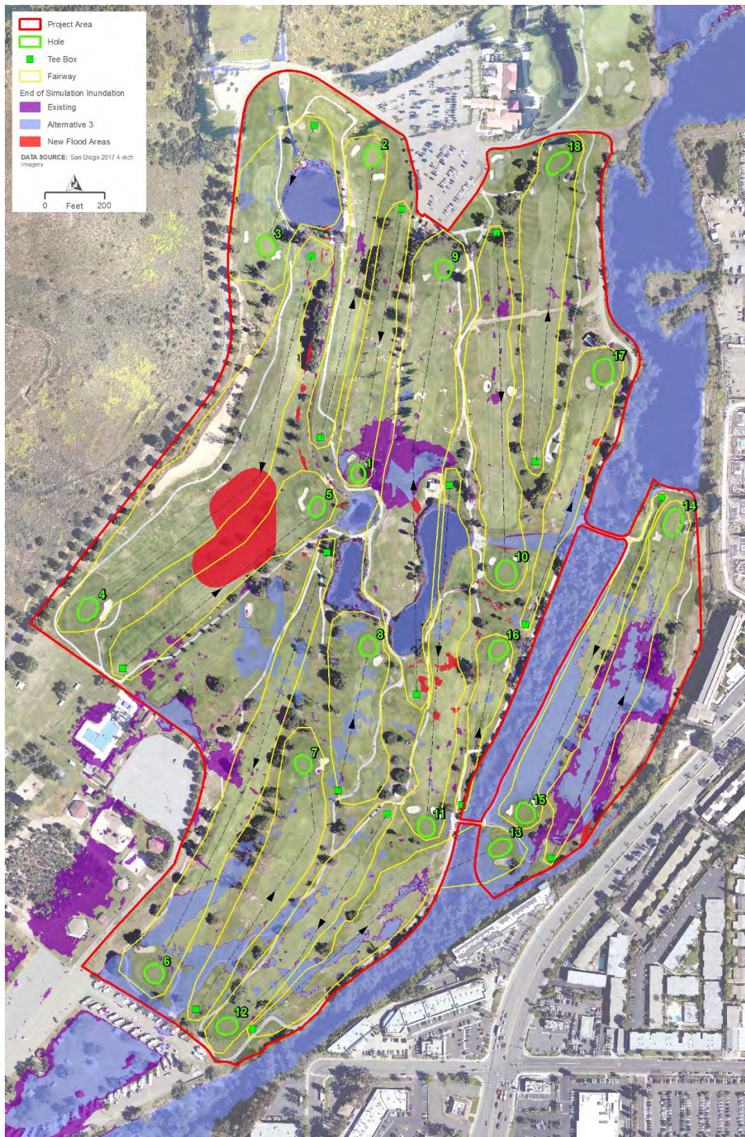
Figure 3-9 Preferred Alternative vs. Existing, North Basin 100-year, Post-Event Inundation
