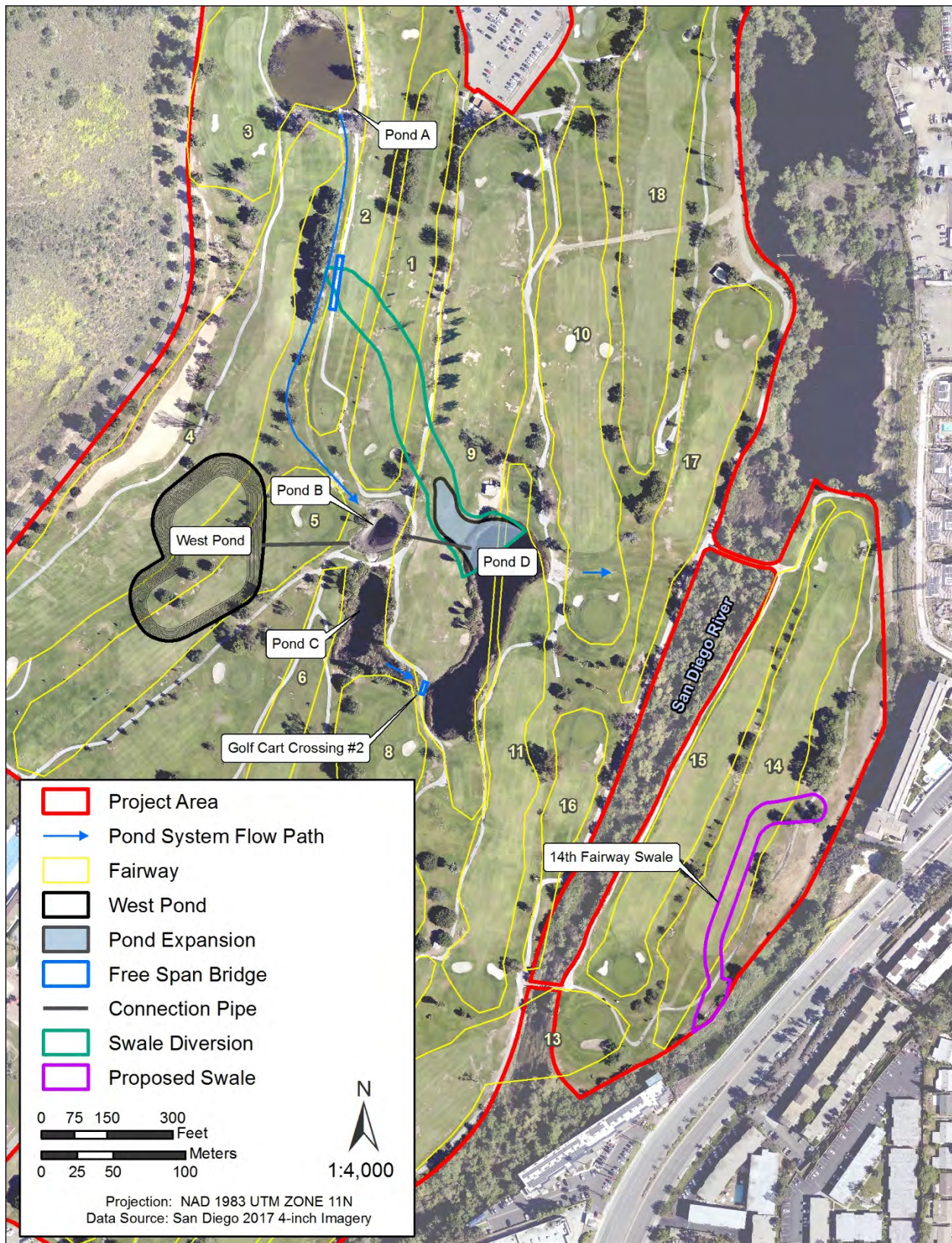
Figure 2-2 Alternative 3 Drainage and Conveyance Features
