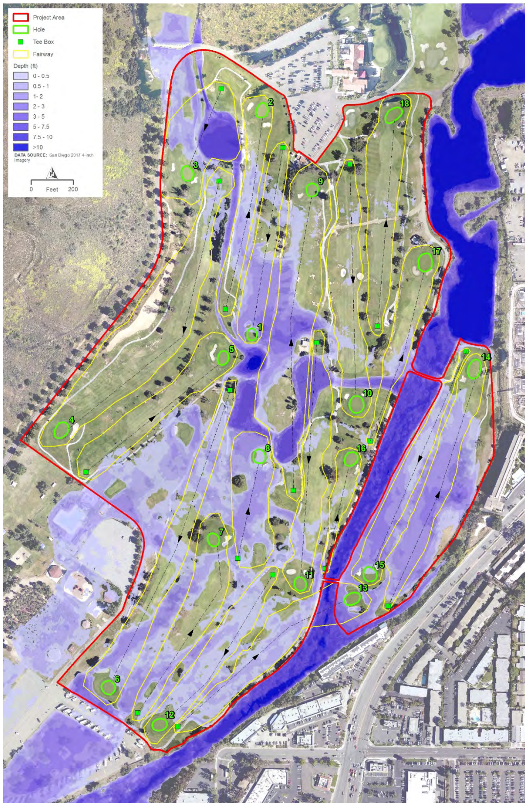
Figure 3-4 Existing Conditions, North Basin 100-year, Maximum Inundation
