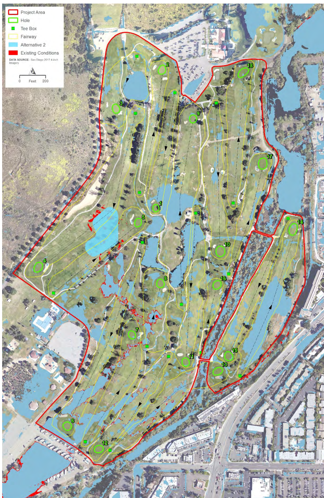
Figure 3-6 Alternative 2 vs. Existing Conditions, West Hills 100-year 24-hour, Post-Event Inundation
