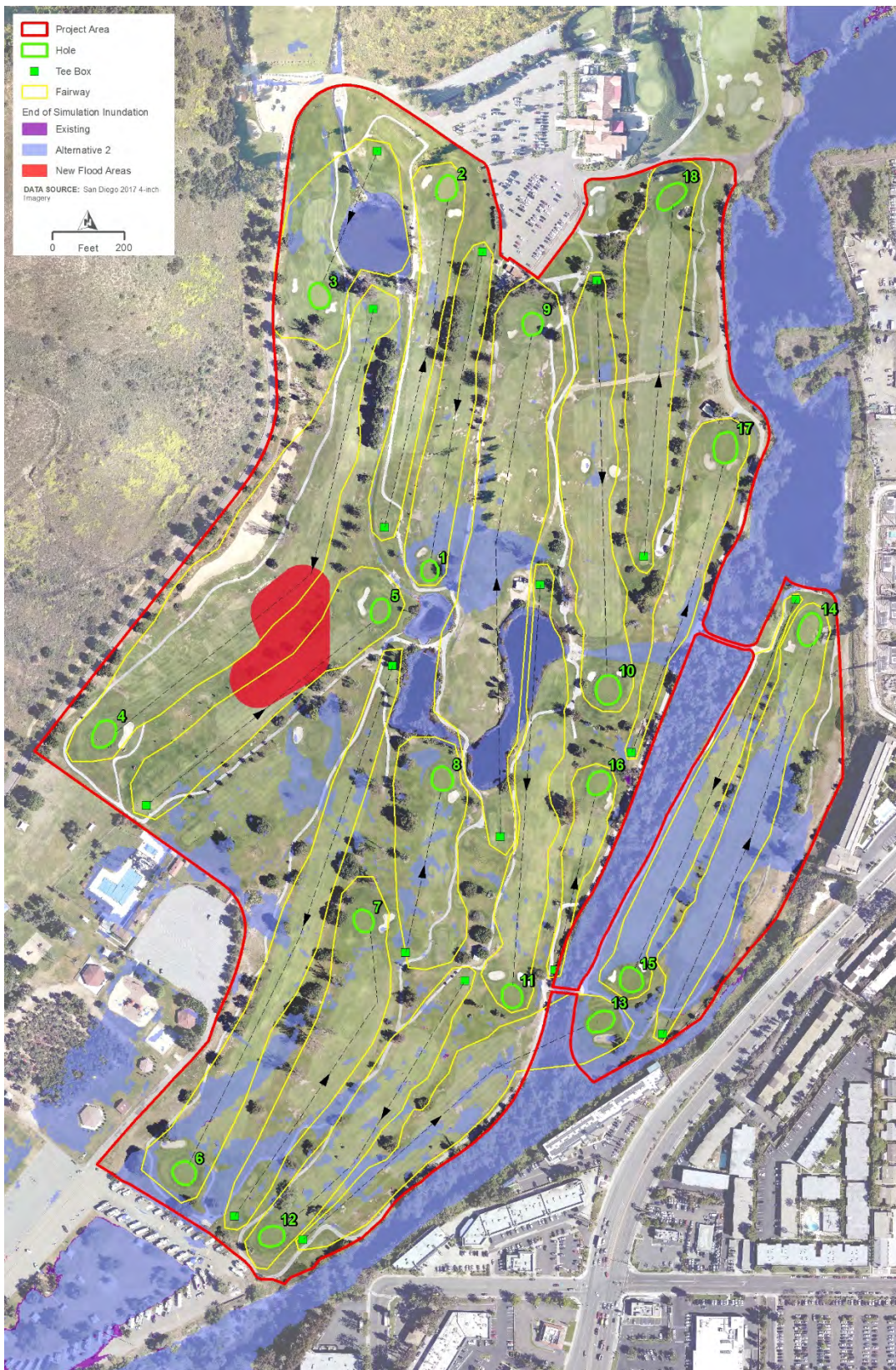
Figure 3-7 Alternative 2 vs. Existing Conditions, North Basin 100-year, Post-Event Inundation
