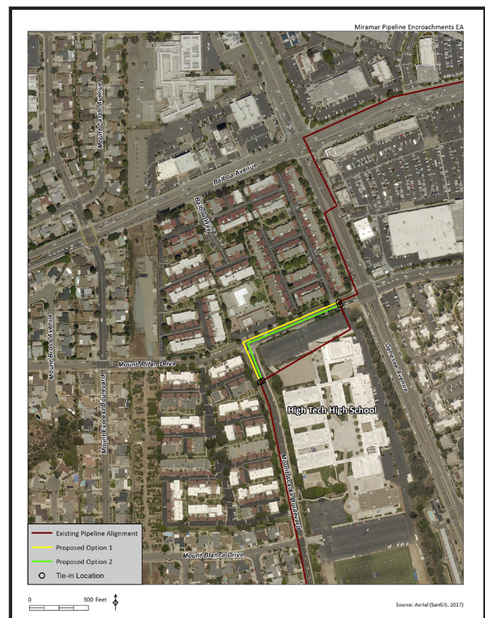
Figure 2 – Encroachment at High Tech High: Proposed Options 1 and 2 for Pipeline Realignment to Address High Tech High Encroachment.
